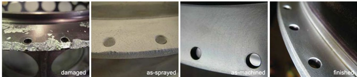
Figure 4. Consistent corrosion on the flange.
