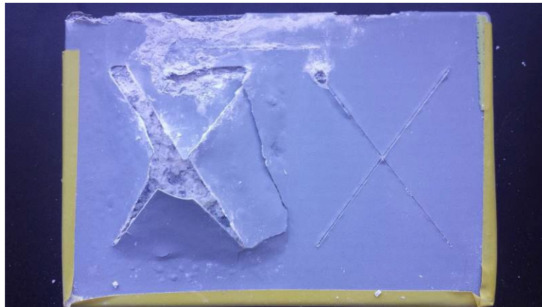
Figure 9: Corrosion panel after 500hrs acidified salt fog, (left) magnesium prime/paint only, (right) magnesium 6061 CS, prime/paint.
