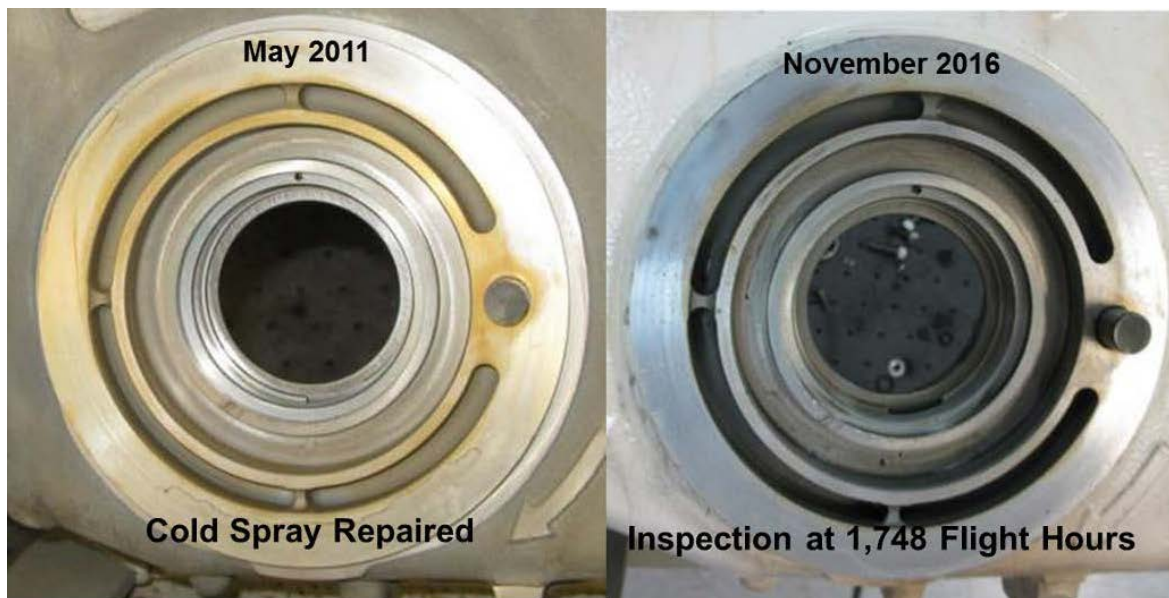
Figure 13: Aluminum housing inspection after 1,748 flight hours.
