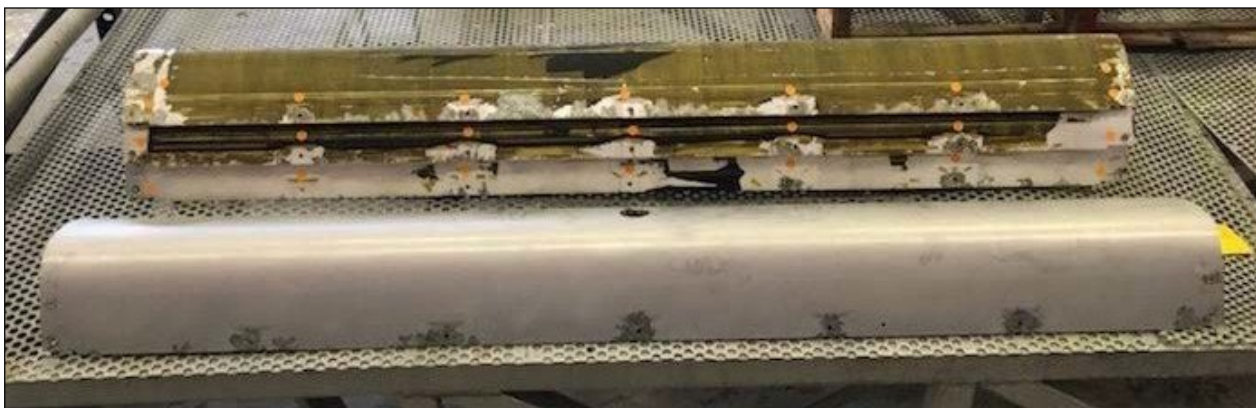
Figure 14: Corroded areas on leading edge around lower fasteners.
