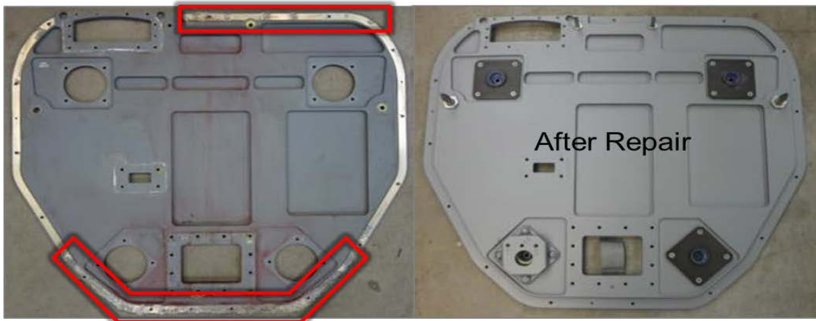
Figure 11: Avionics rack repair.
